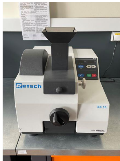
Figure 2 Laboratory-grade jaw crusher with tungsten carbide crushing jaws
