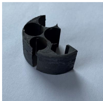
Figure 3 Leftover sintered preform after ED machining
