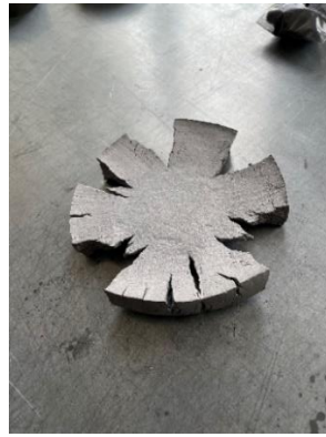
Figure 1 Result of a failed sintering densification of MAX phase (about 600g of material)
