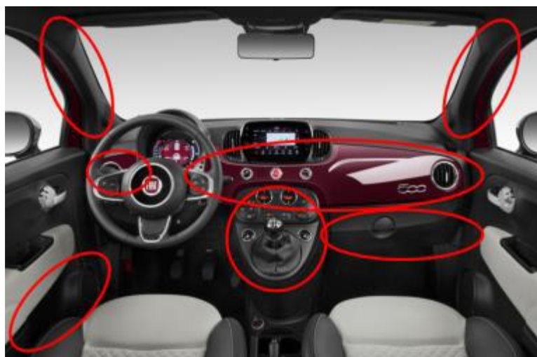
Figure 3: Automotive interior parts to be modified by renewable composites produced during the SSbD4CheM project.
