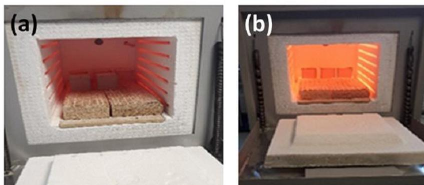
Figure 57: The used laboratory electric furnace in operation, at (a) 800 °C and (b) 1050 °C
