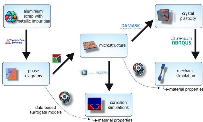
Figure 28: Schematic workflow for digital twin creating including utilized software packages.
