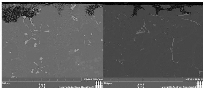
Figure 29: SEM of cross-section after potentiodynamic experiment of artificially impurified AlSi7Mg0.3 with (a) 1.0% Fe, 0.6% Cu, 0.6% Mn and (b) 0.5% Fe, 0.05% Cu, 0.2% Mn
