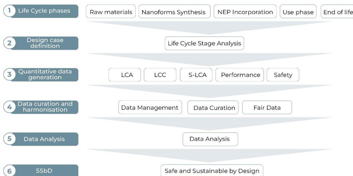
Figure 17 General view of data generation from each Life Cycle Phase towards the generation of the Safe and Sustainable by Design solutions by the INTEGRANO Decision Support Tool.
