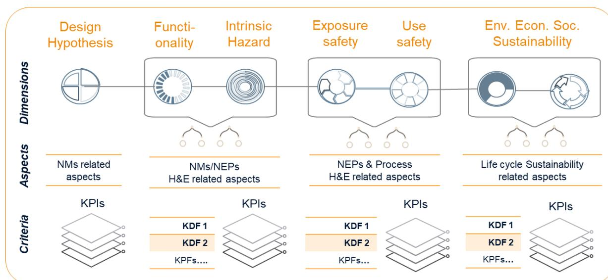
Figure 44. Dimensions, aspects and criteria of the SSbD framework, following a hierarchical approach in which functionality & safety aspects are considered first, followed by process related safety and environmental sustainability and economic aspects, while assuring product functionality. The SSbD approach within ASINA captures Key Performance Indicators (KPIs) in each dimension, Key Decision Factors (KDFs) and Key Performance Factors (KPFs).
