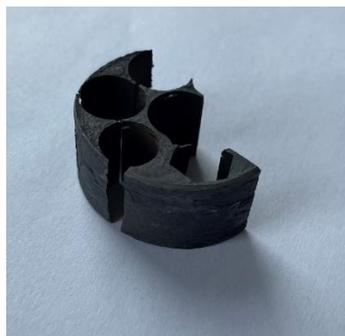
Figure 3 Leftover sintered preform after ED machining
