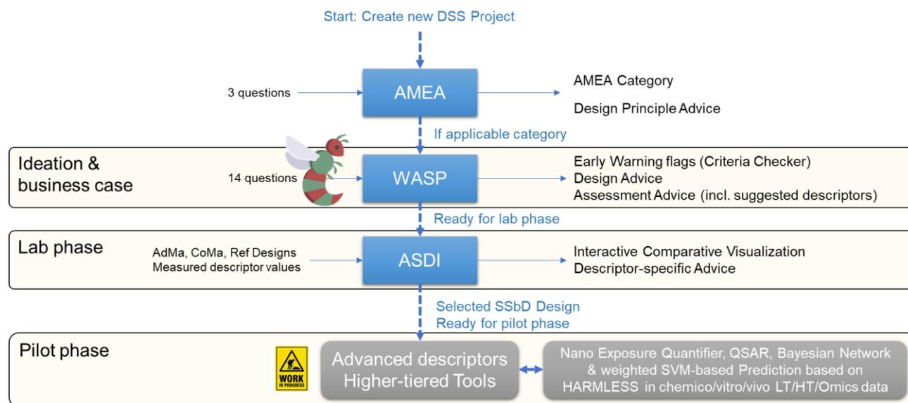
Figure 42: Improved workflow of the DSS: AMEA = Advanced Material Earliest Assessment, WASP = Warning flags, design Advice, Screening Priorities, ASDI = Alternative SSbD Design Inspector.
