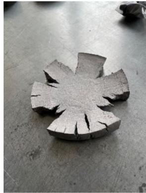
*Figure 52 Result of a failed sintering densification of MAX phase (about 600g of material)*
