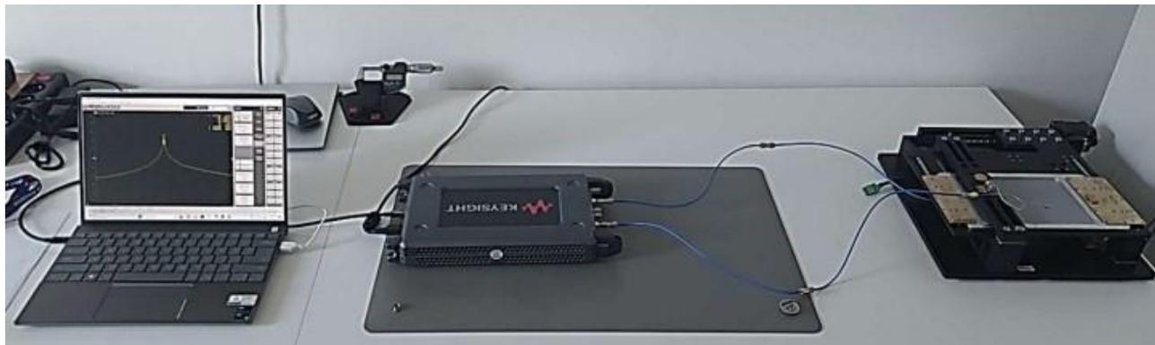
*Figure 1: Measurement setup for imaging the electrical parameters of the tested material using a 10GHz iSiPDR scanner*
