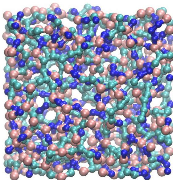
Figure 24: Typical amorphous structure of aBN:C compounds, namely an amorphous BN structure with a certain density of carbon atoms, affecting the overall system properties (thermal stability, mechanical and dielectric properties, etc)
