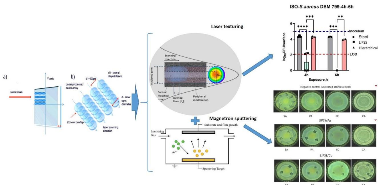
Figure 64: Effects of femtosecond laser texturing and and postmodification with magnetron sputtering and visualisation of bacterial assays and screening touch test performed on laser structured (in the form of LIPSS) magnetron sputtered samples with Ag and Cu. SA : *S. aureus* ATCC 6538P, PA: *P. aeruginosa* ATCC 15442, EC: *E. coli*, ATCC 8739, CA: *C. albicans* DSM11225
