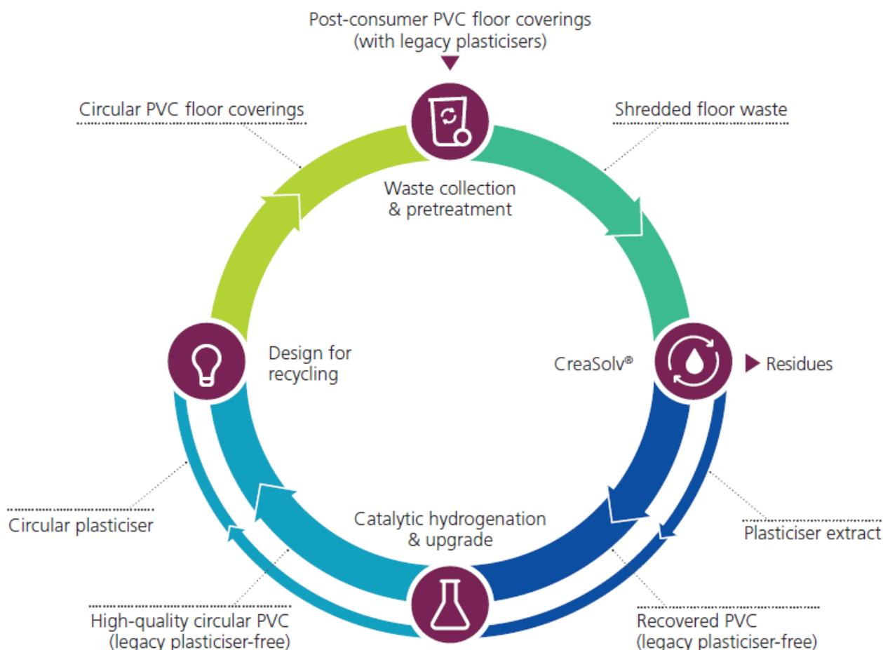
Figure 65: The recycling process
